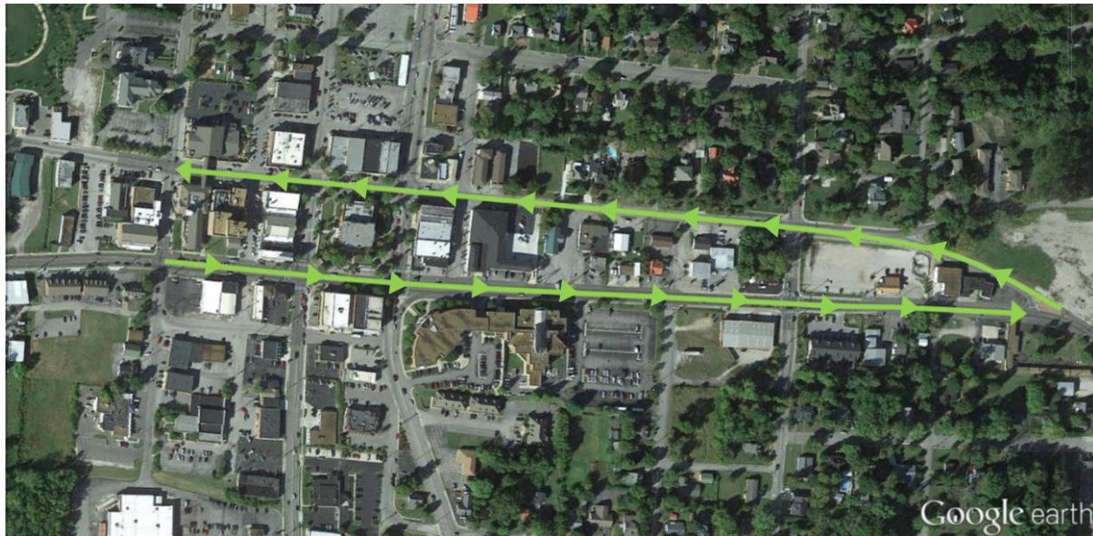
Figure 19: One-Way Pair Lane Configuration at Jefferson Avenue and Washington Avenue
